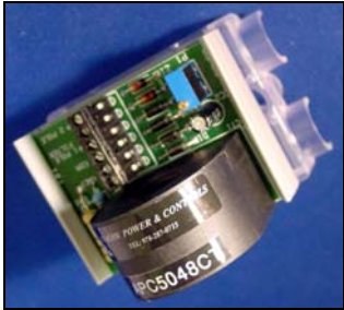
APC5048CT Current Transformer Module
